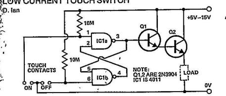
The cost of many CMOS ICs is now lower than a mechanical on/off switch Using only one half of a 4011, plus a couple of general purpose transistors, a touch operated switch can be constructed which is ideal for many battery powered projects
